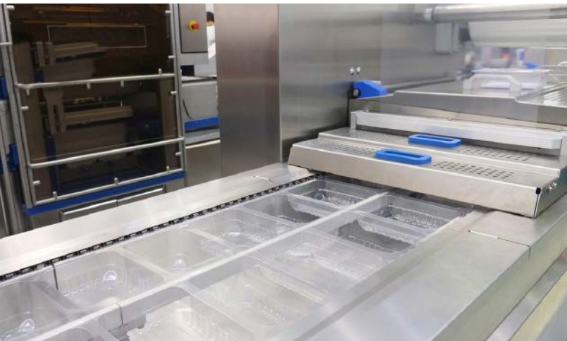
The AC servo drives precisely position two set of axes for the following placing and packaging by conveyors
