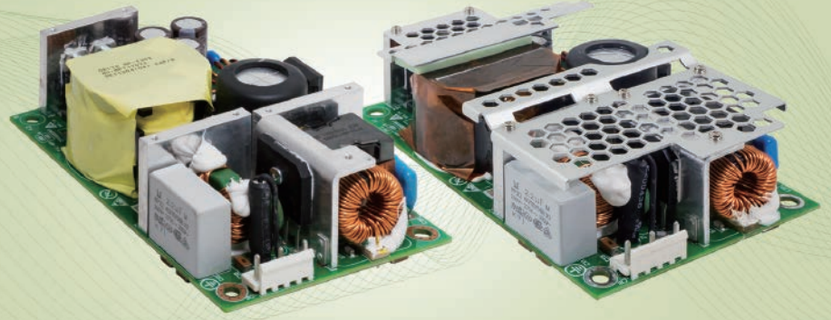
Delta's newest PJP series of open frame power supply for lighting applications
