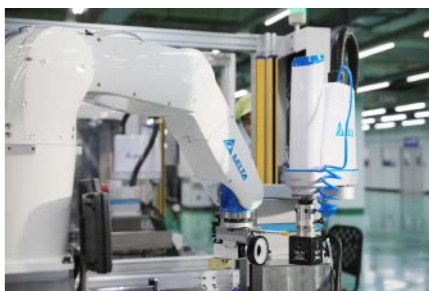
The DRV70L Series completes SCARA robot function tests on Delta's production line to reduce manpower, shorten testing time, and enhance testing efficiency
