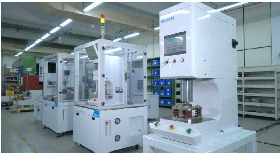
Delta develops and manufactures all the key components of the servo press (including PLCs, servo drives, motors and an HMI) for seamless integration and stable performance
