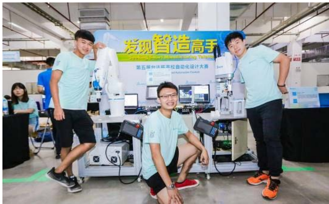
The team from National Kaohsiung First University of Science and Technology adopted both Delta's SCARA and Vertical Articulated Robots to build the solution of a unmanned robot workstation, achieving an optimized process of high-precision manufacturing
