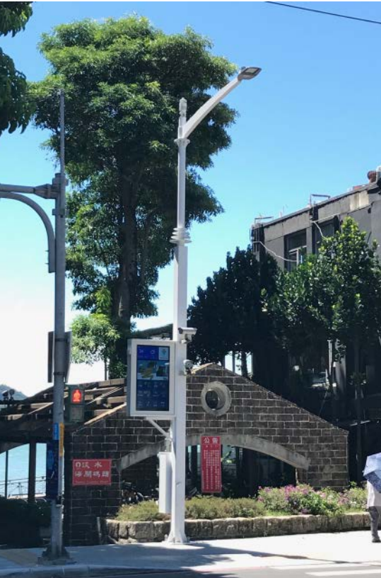
Delta's Smart Street Lighting Solution provides environmental sensing which gathers the city's day-to-day data such as temperature and humidity, wind direction, wind speed, and more, to be used as parameters for controlling smart lighting
