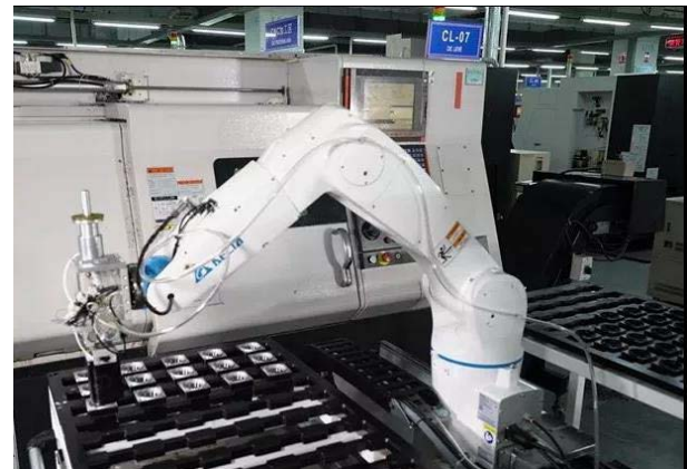
Delta's automation solutions assist in automatic loading and unloading of machine tools to improve efficiency
