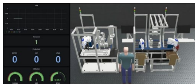
Digital twin technology is used to simulate product design, smart adjustment of the machine, production line configuration, etc.
