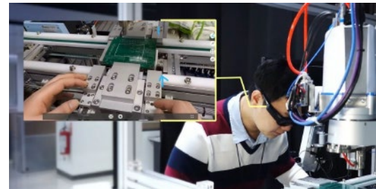
On-site personnel wear AR glasses and connect with remote experts online in a real-time manner to perform maintenance of the machine
